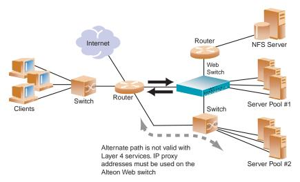
Figure 6-4 SLB Client/Server Traffic Routing
